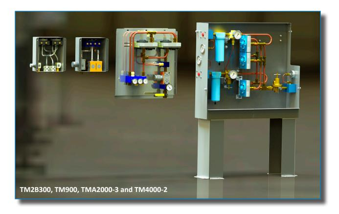
McDantim **Trumix®** gas blending systems are all based on a unique approach to creating accurate gas blends. Taking advantage of laminar gas flow properties, our Blenders maintain industry standard blend accuracies over a wide range of flow rates without the need for buffer tanks, electrical connections, or user calibration. Two-component or three-component blends at flow rates ranging from 1 scfh to over 4000 scfh are available from our range of products.
